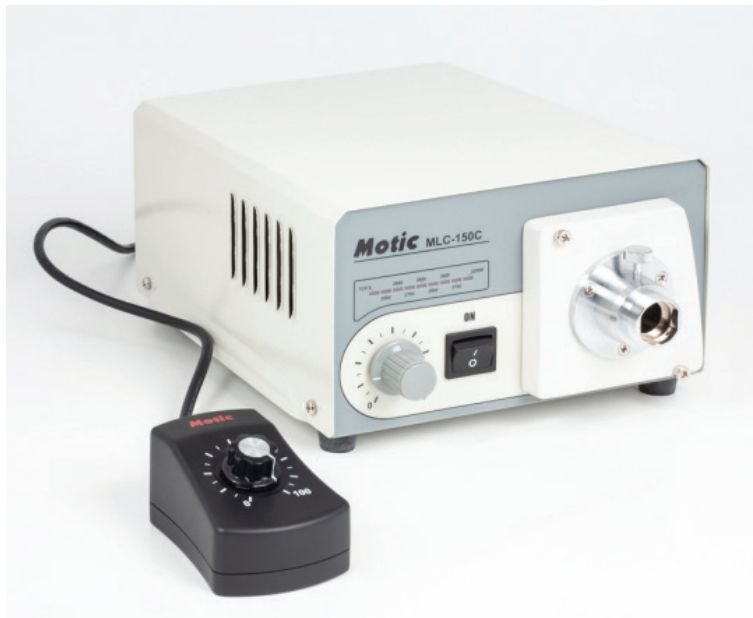
1101002000011 MLC-150 Fiber optic illuminator Halogen illumination 21V/150W (EKE) Power supply 100-240V (CE) Local/remote switch for intensity control 2m remote control intensity Colour temperature LED read out
